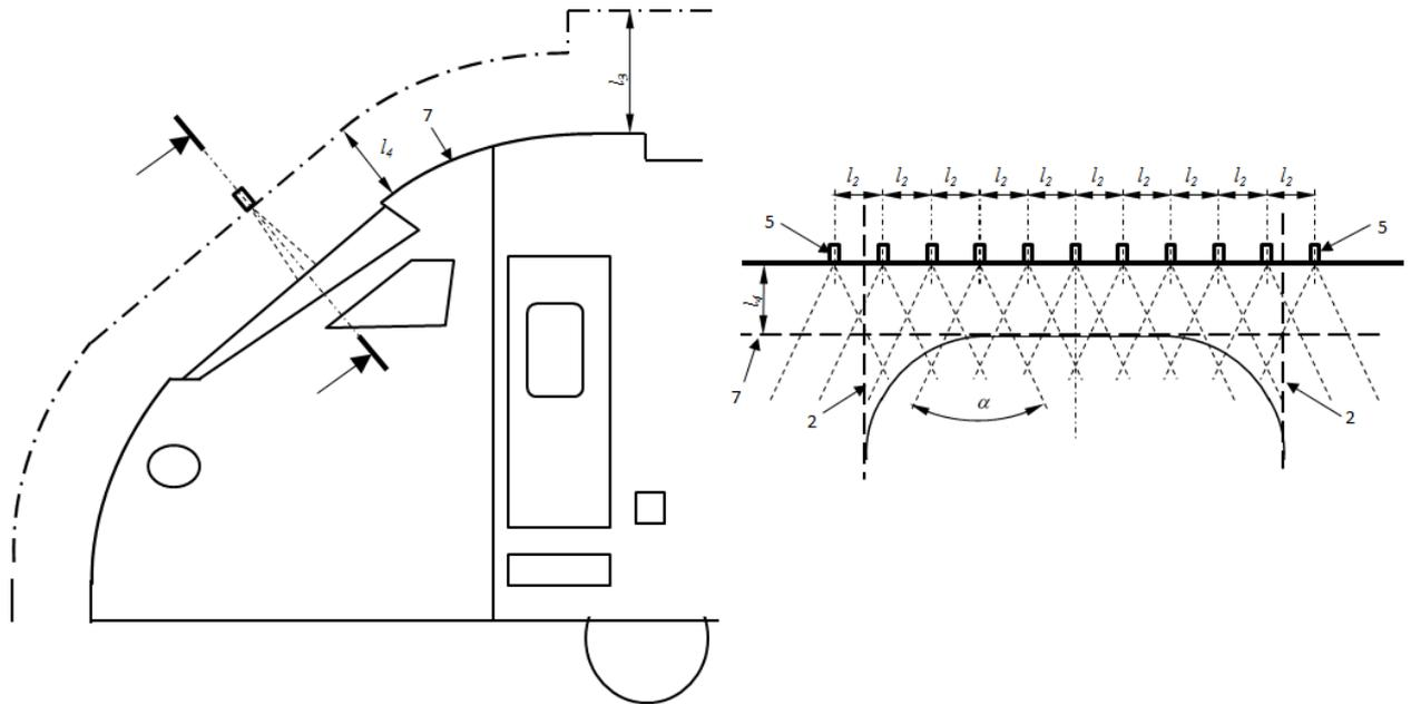
Figure 4 — Water test arrangement
