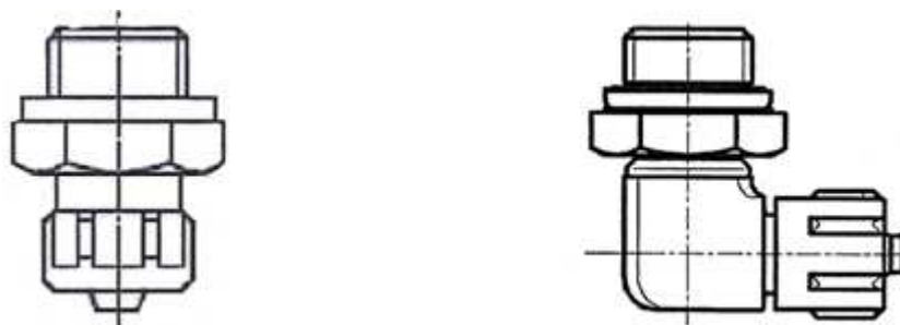
Figure 11 – Air fittings possible shape
